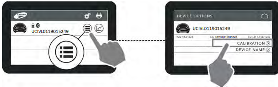
Figure 21 – Calibrating the Urocap™ IV Light
